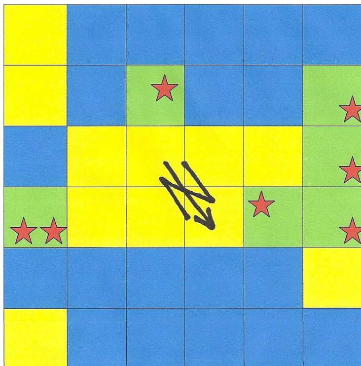
Figure 10: Samedan helipad, condition of the 36 gratings (G) after the incident on 8 October 2009
