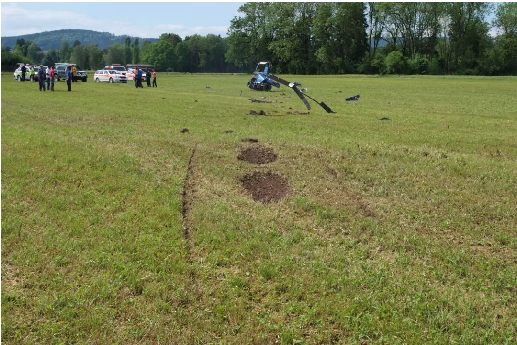
Figure 2: In the foreground, the initial traces of impact of the skids and the underside of the fuselage can be seen, further back is one of the two main rotor blades, which was torn off and which stuck in the ground, the main wreckage can be seen to the rear.
