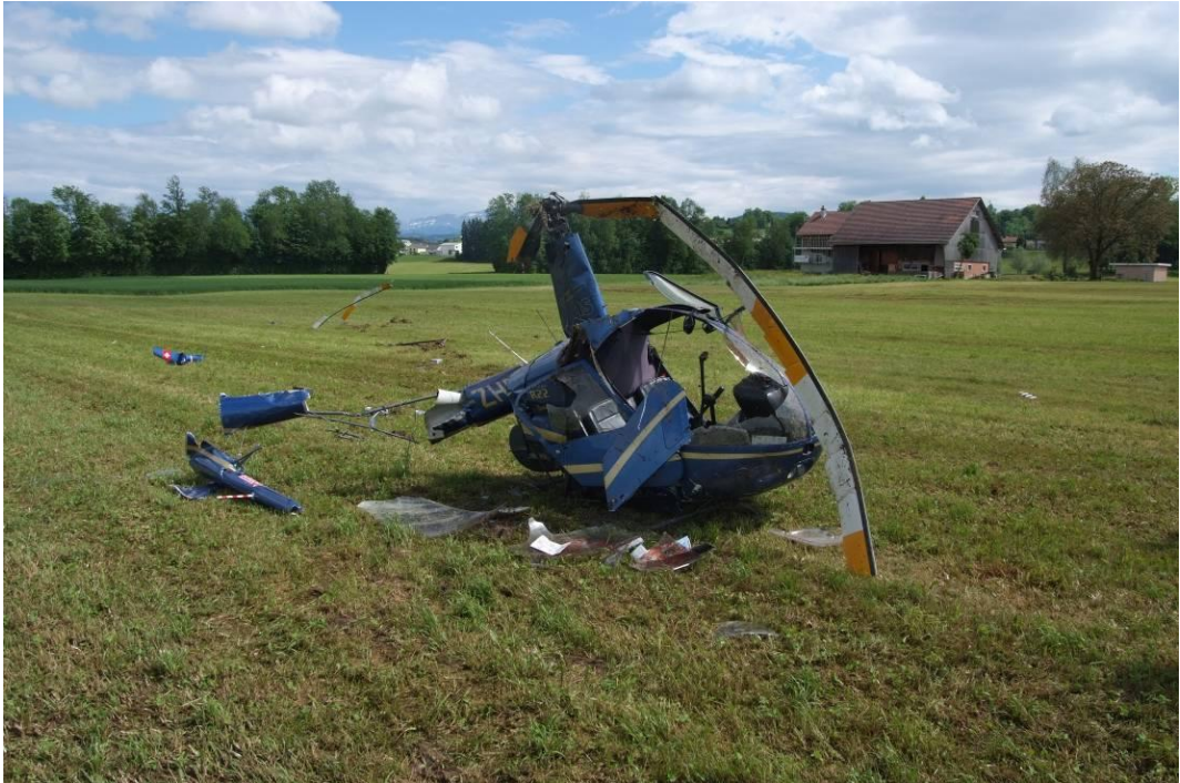
Figure 1: Main wreckage of the helicopter after the accident. The helicopter was righted after the accident to prevent further leakage of fuel, oil and lubricants. In the background, other individual components and various traces of impact can be seen, allowing the direction of approach to be determined (approximately the reverse of the camera angle).
