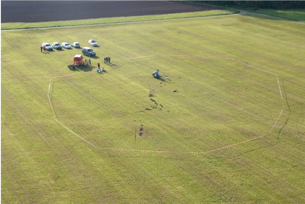
Figure 3: Initial impact traces, other impact traces and individual components, plus the main wreckage, photographed from the air from the approximate direction of approach.
