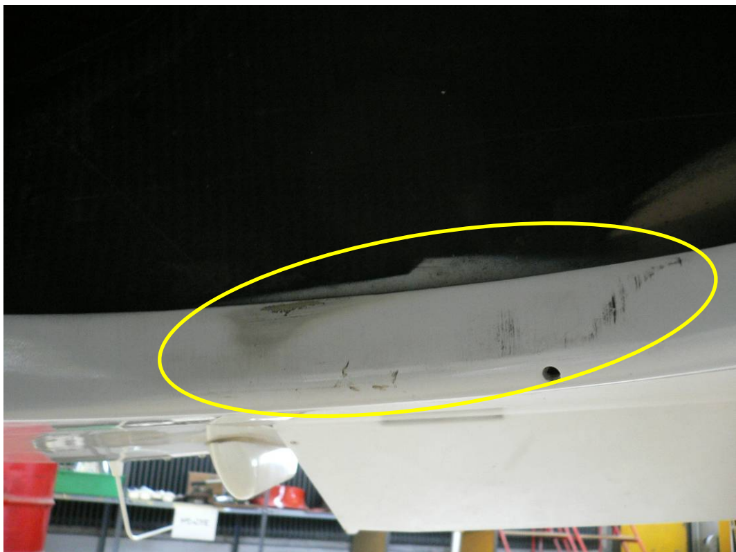
Figure 6: Remaining scratch marks after the tyre marks were cleaned off
