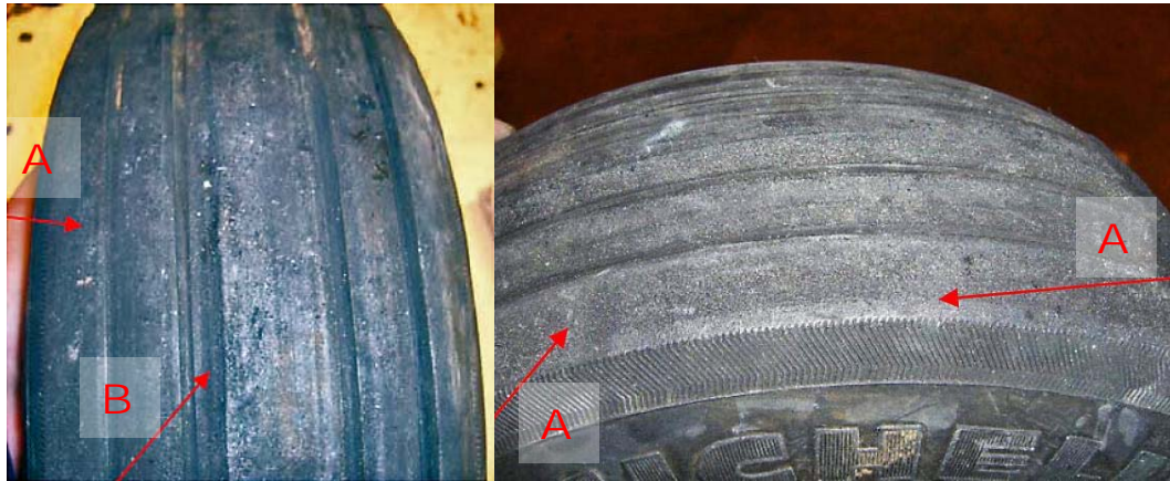
Fig. 10: Worn down tread of right tyre (A= worn outboard shoulder; B= Groove on the bearing surface)
