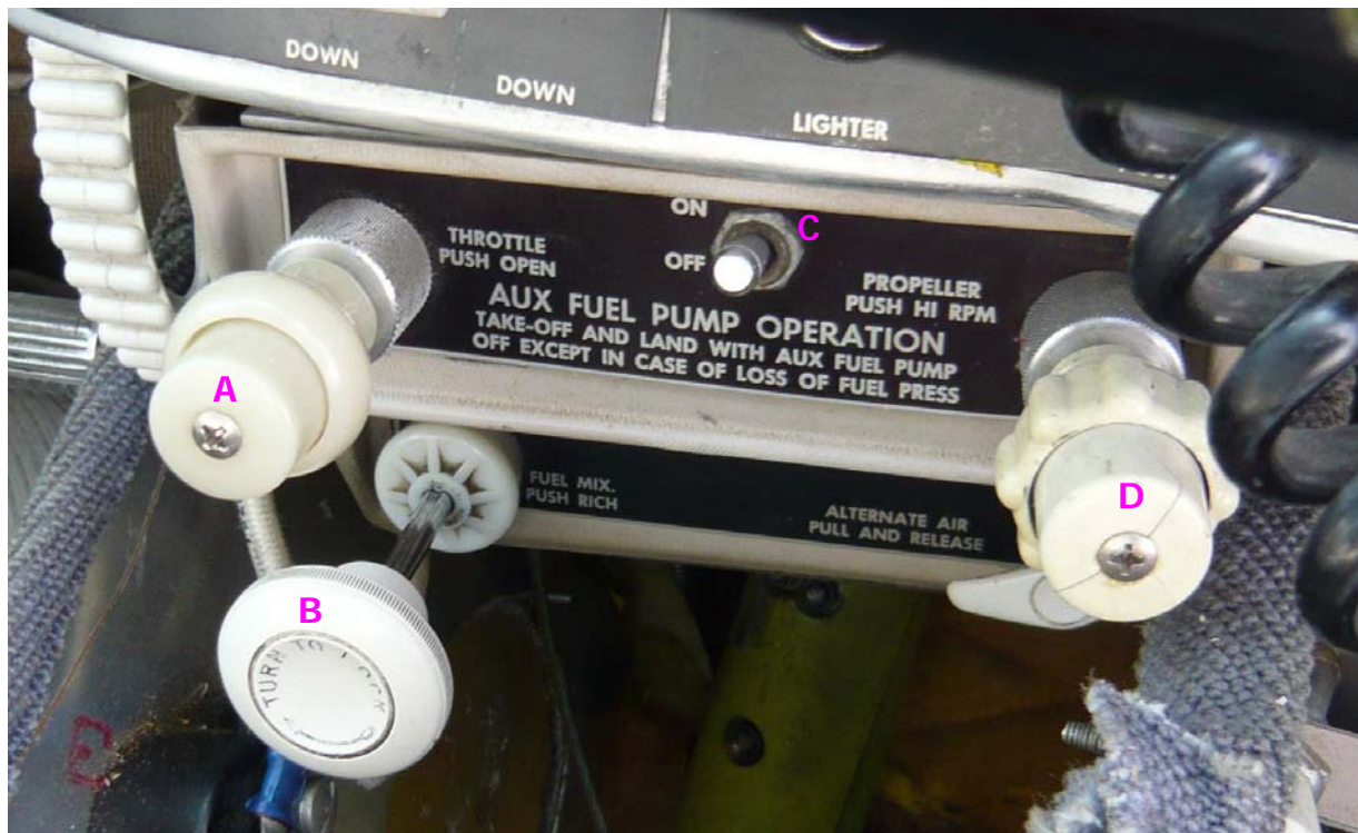
Annex 1 - Position of the controls after the accident
