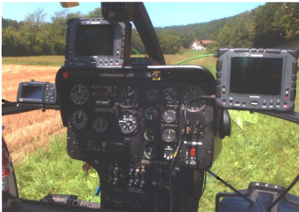
Figure 7: View from cockpit, Garmin GPS seen pilot side left, one camera monitor each for pilot and director.
