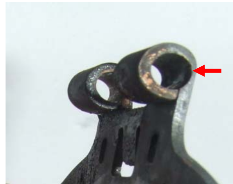
Fig. 2: Wear on the float hinge
