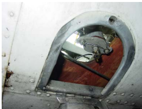
Fig 2: Main drain located under the floor of the cabin.
