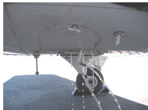
Fig 3: Fuel leakage from the main drain with engine shut down
