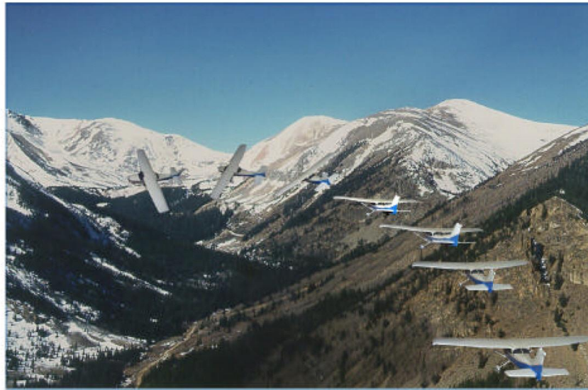
STEEP TURN COURSE REVERSAL – Simultaneously begin bank, add power and extend flaps.
