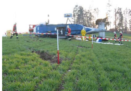
Fig. 5: Initial traces of contact of the rear landing gear with the terrain
