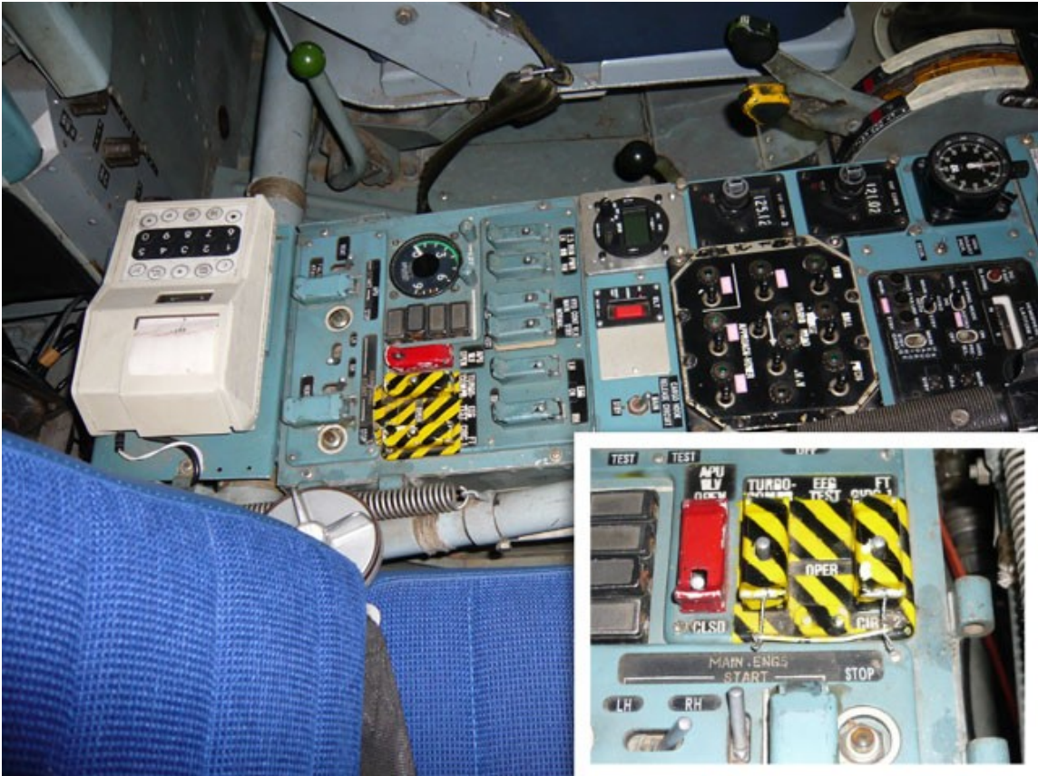
Centre console after the modification from the viewpoint of the pilot in the right-hand seat. The enlarged extract shows the detail of the modification.
