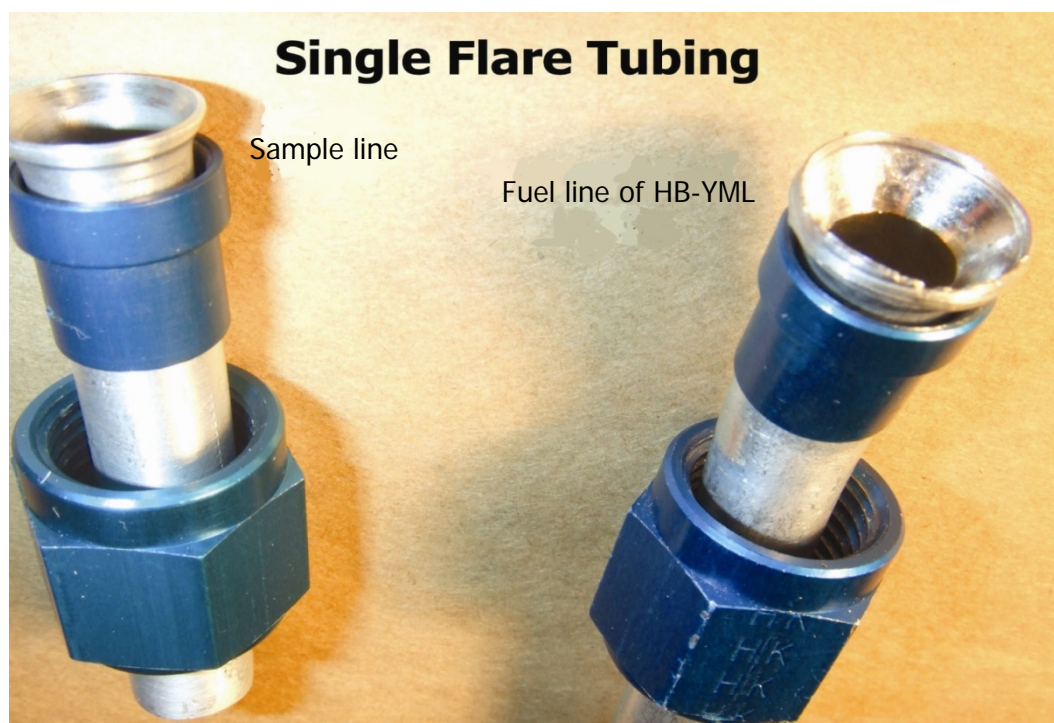
Fig. 7: Left: line with correctly fabricated flare, right: line from aircraft HB-YML with a flare not fabricated according to norm SAEJ533
