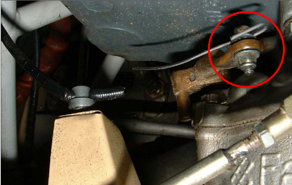
Fig. 1 Mixture control, incorrect assembly
