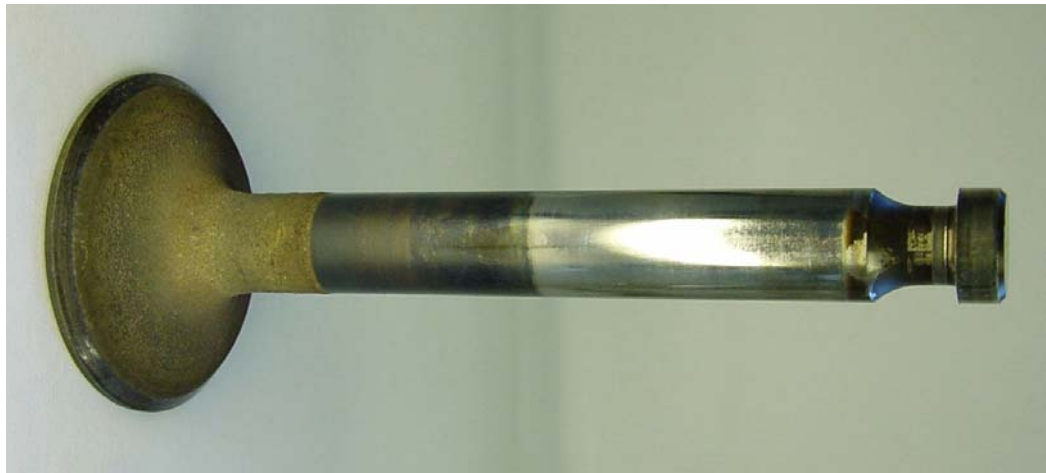
Cylinder No. 3 exhaust valve with deposits on the lower part of the valve stem
