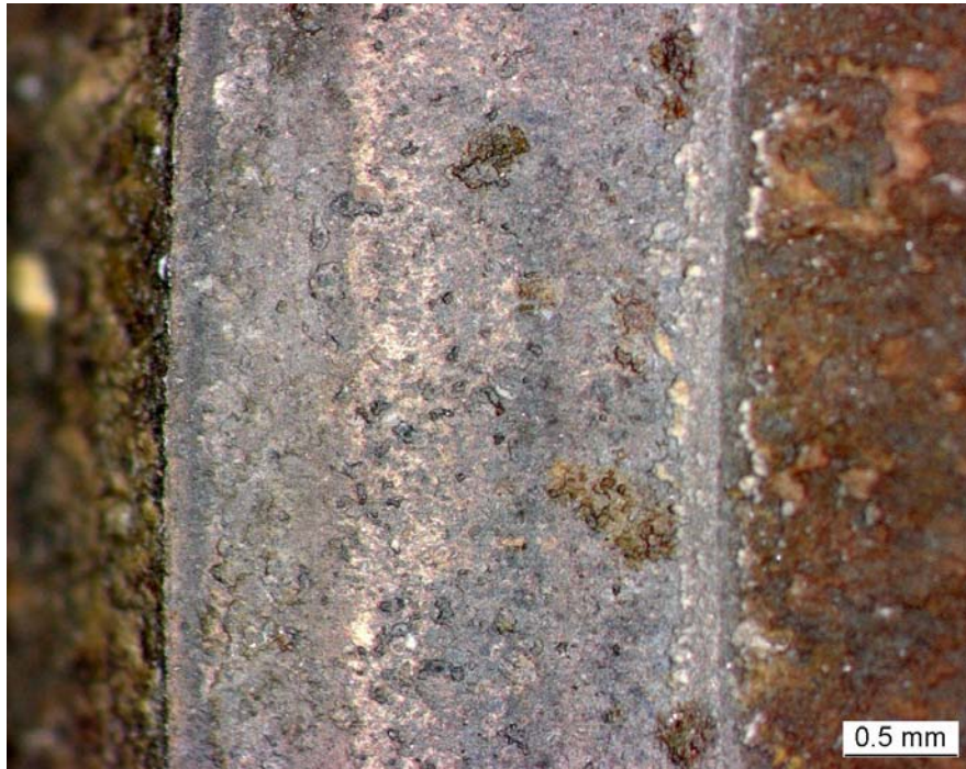
Carbon residue on the fit of cylinder No. 3 exhaust valve
