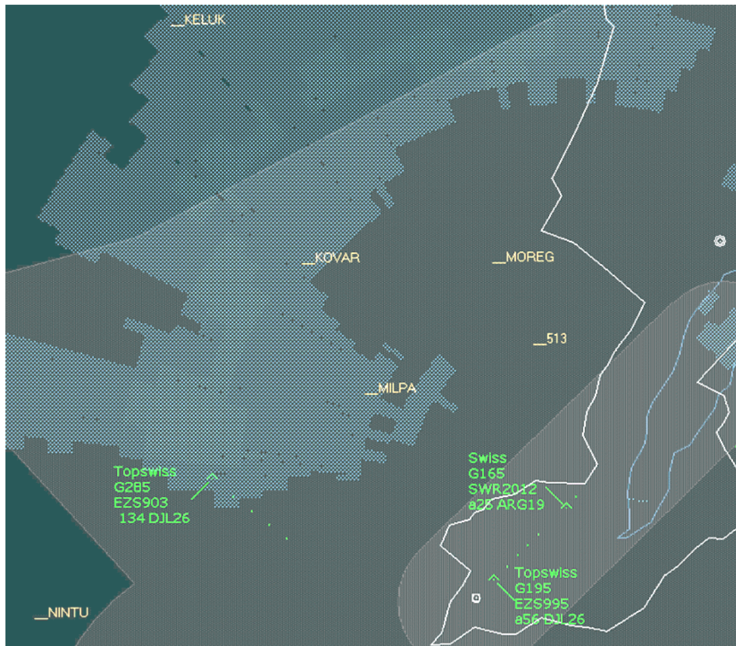
Fig. 4 Representation of part of the ASR10SS radar image as it would have appeared on the ICWS console at 08:00:01 UTC.
