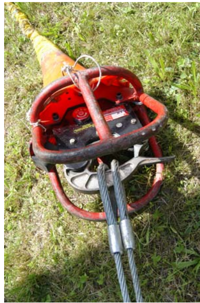
Figure: Lower cargo hook with two suspended “choker cables”
