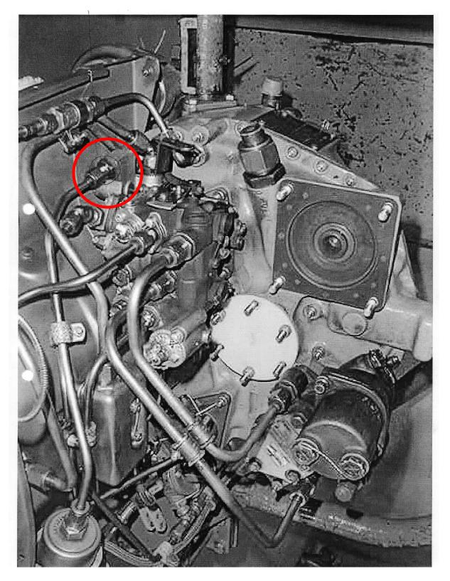
Annex 2 Torque paint (slippage marks) on the "B" nut after tightening to the correct torque value
