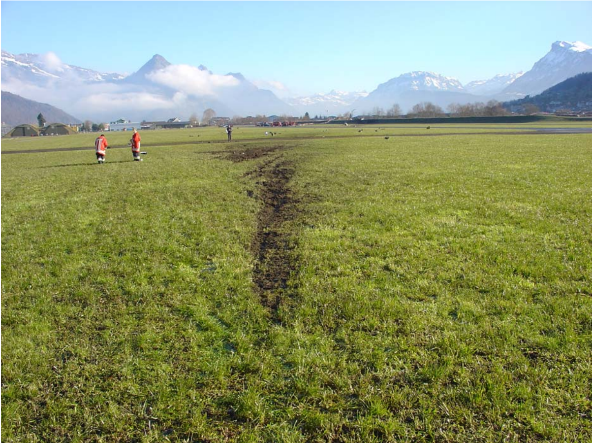
First traces of right wing impact
