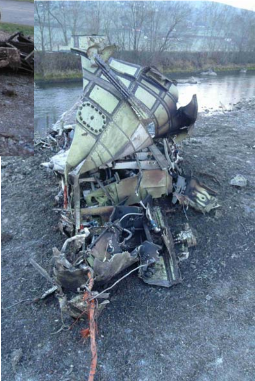
Final position of wing main- spar / fuel tank section
