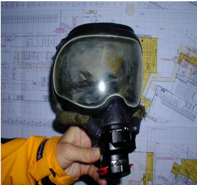
Copilot's heavily contaminated full face mask screen
