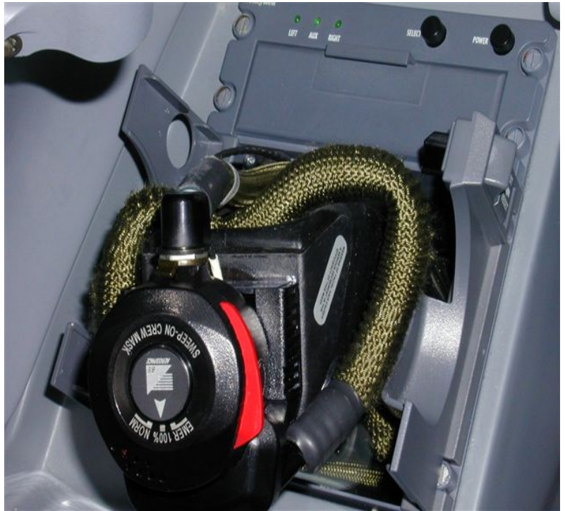
Oxygen mask, halfway pulled out of the "stowage box"
