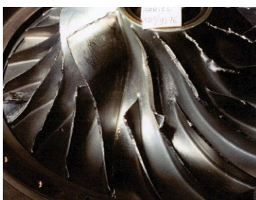
Centrifugal compressor wheel: one blade broken
