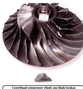
Centrifugal compressor wheel: one blade broken
