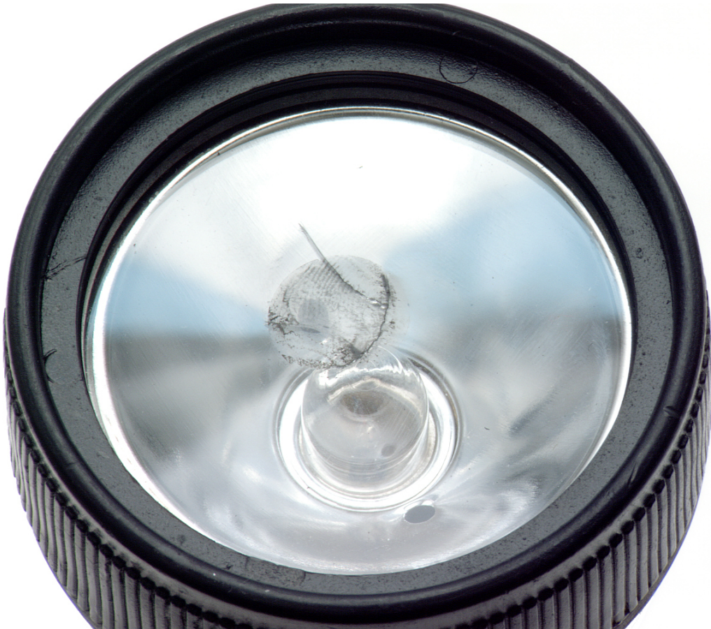
Fig. 1 Lens of Torch lamps with melted plastic
