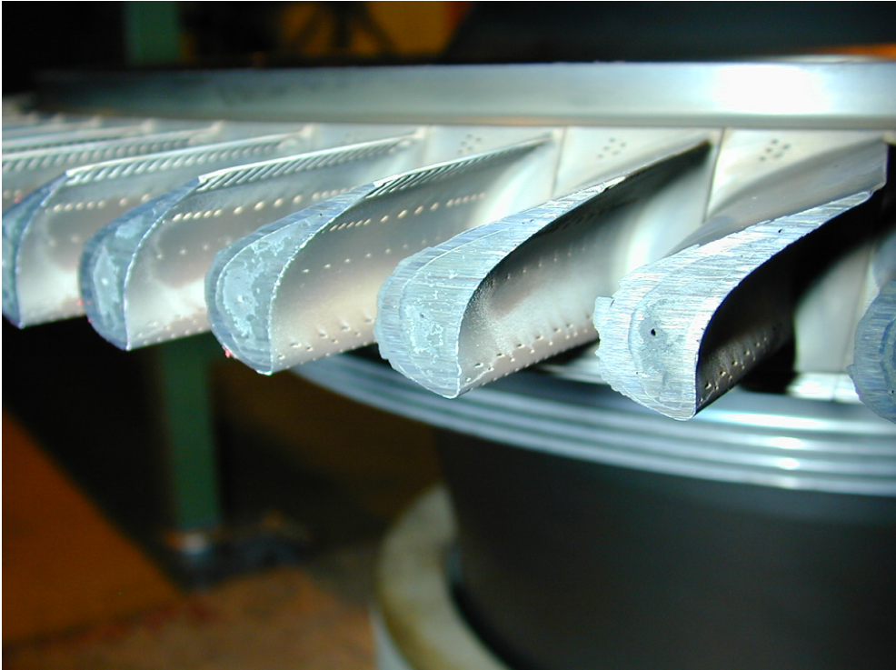
Fig. 4 Damaged blade tips
