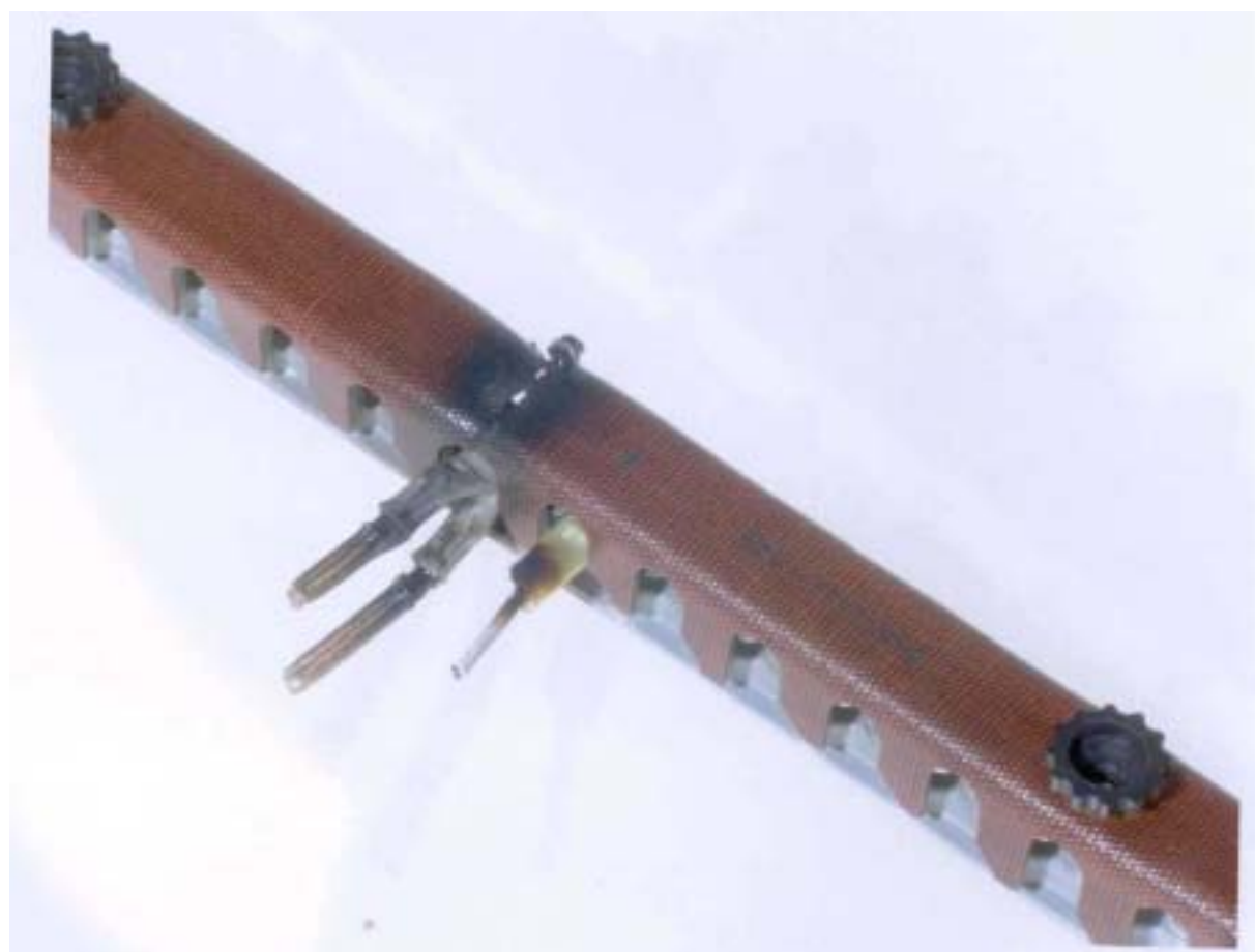
Fig. 2 Terminal Board with heat damage
