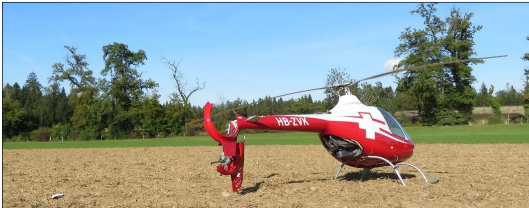
Figure 2: Final position of the HB-ZVK helicopter looking north-east with a detached enclosed tail rotor.
