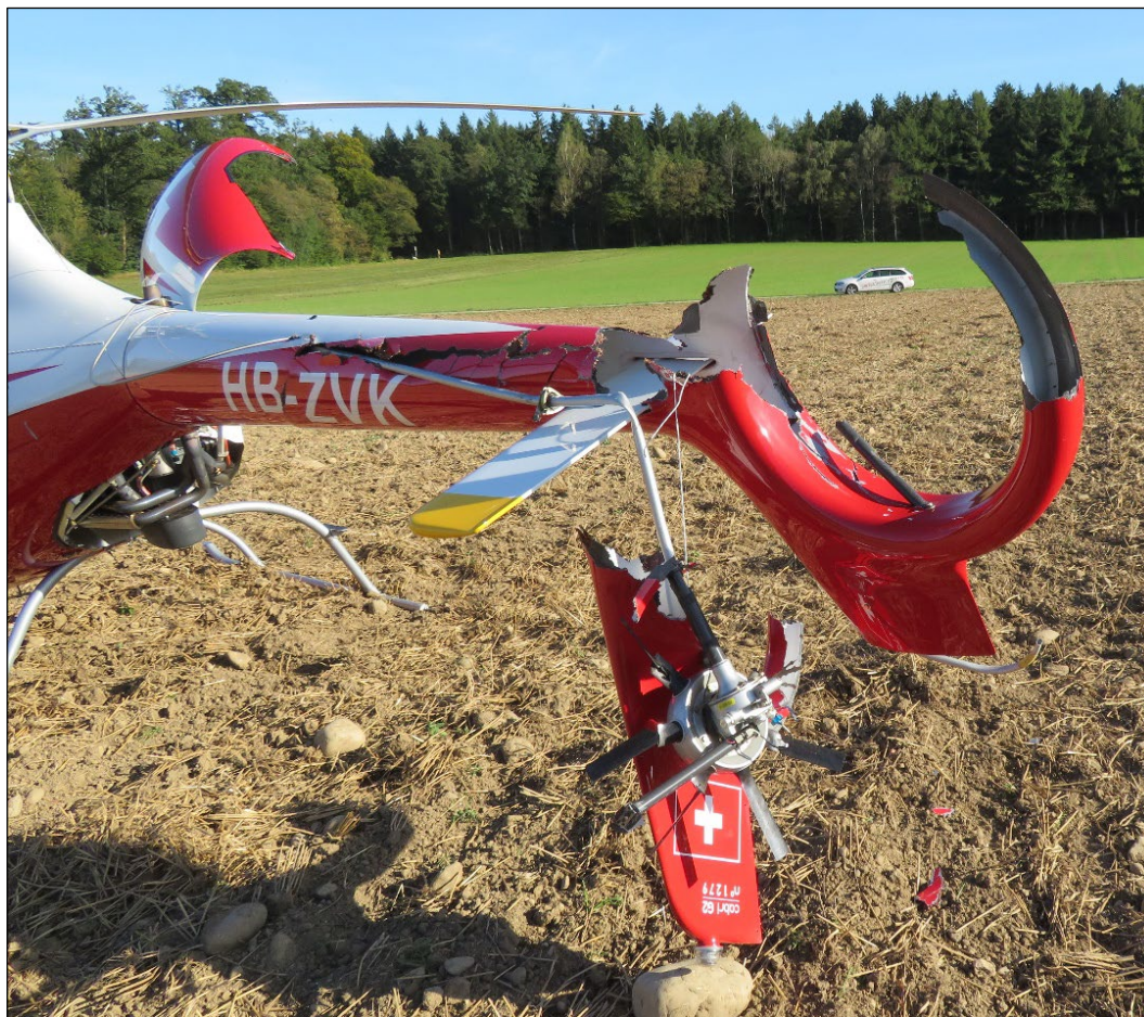
Figure 5: The HB-ZVK's destroyed tail boom with the tail rotor torn out
